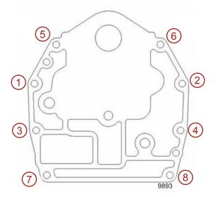
F25-60 Powerhead Bolt Torque Sequence
