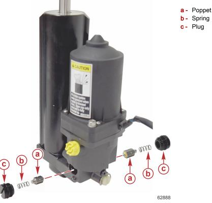
2. Replace the power trim up-circuit/tilt pressure relief valve (poppet) as outlined in the kit supplied service instructions.
