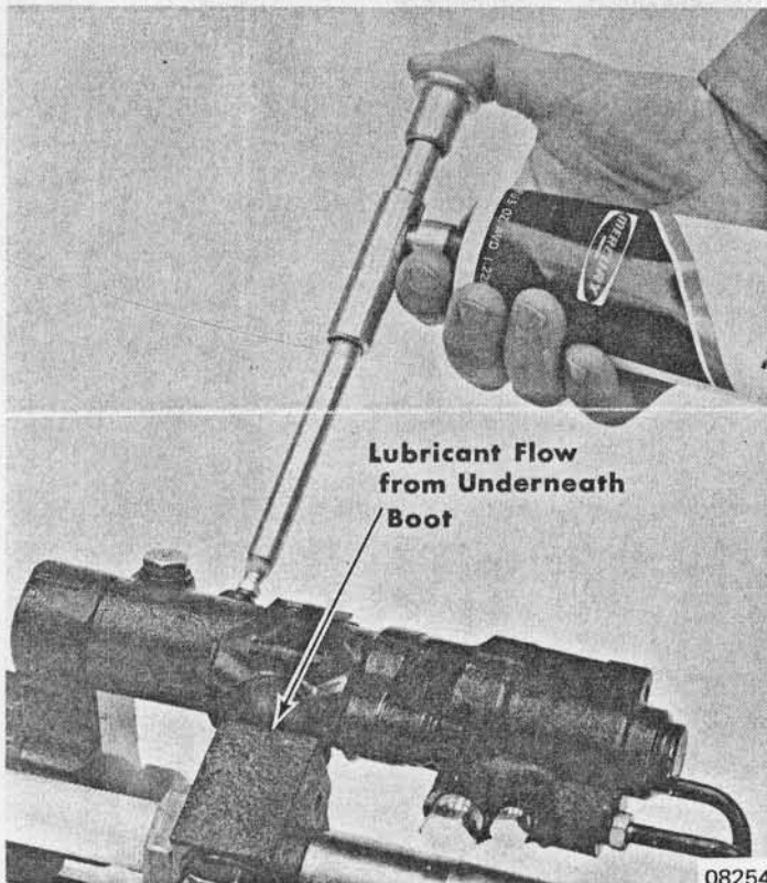
← Figure 5. Control Valve Lubrication
