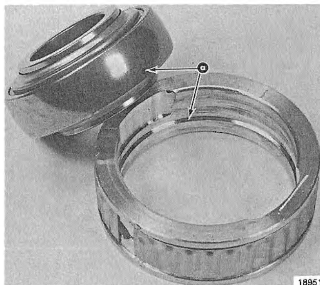
a - Hole In Bearing Must Align With Groove in Cartridge
