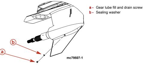
6. Remove the oil vent screw and sealing washer. Allow the gear lube to drain completely.
