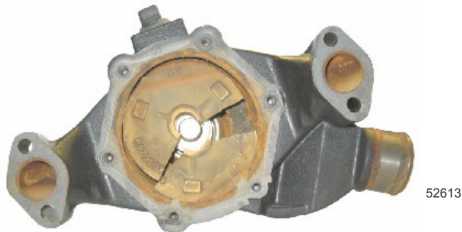
Cracked circulation pump impeller
