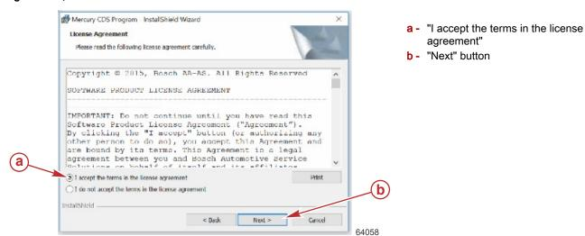
After clicking the "Next" button, the file path where CDS will be installed is displayed. Click on the "Next" button to continue.
