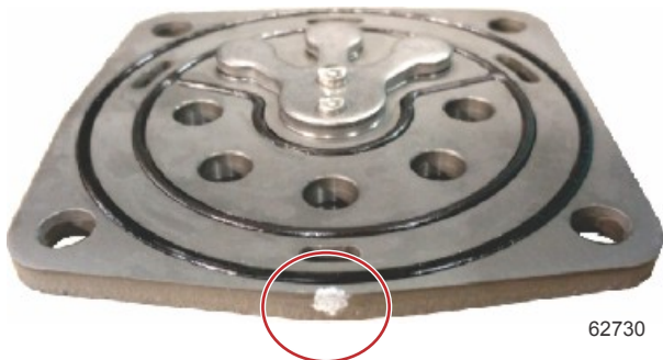
Reed plate assembly edge marked with a white dot
