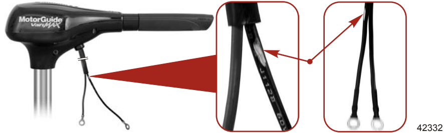
A white mark on the black power cable indicates a replacement top housing
