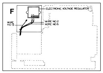
ohmeter across terminal ends of Wires <u>6</u> and 5. Meter needle should indicate Stator Excitation winding resistance, as follows (plus or minus 10%):-
